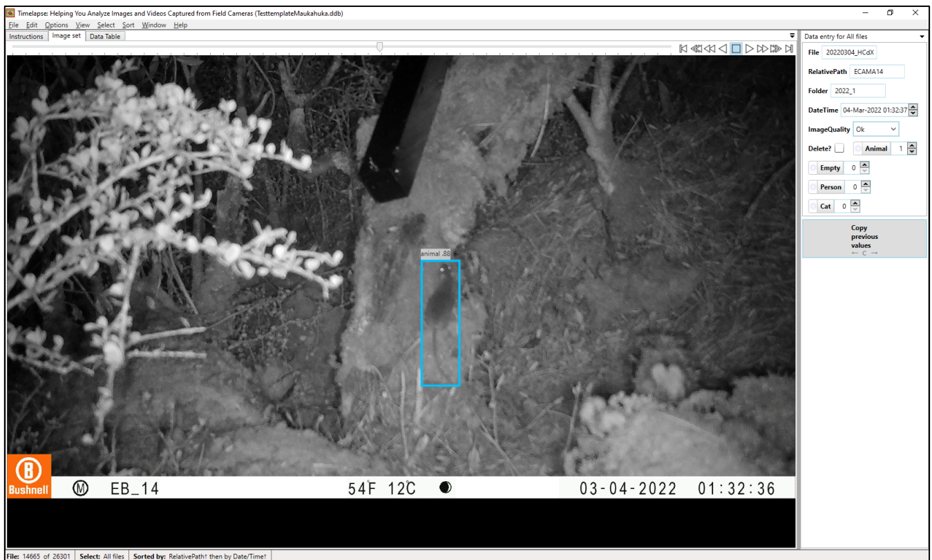
Figure 2: Timelapse2 interface, used in conjunction with MegaDetector to review batch outputs of object detection
